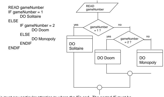
We must pay particular attention to where the IFs end. The nested IF must be <u>completely</u> contained in either the IF or the ELSE part of the containing IF. Watch for and line up the matching ENDIF.
