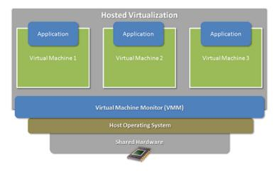
Figure 1. Hosted virtual machine monitors install on top of an underlying host operating system (OS).
