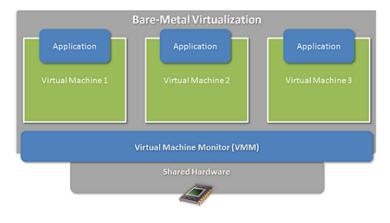
Figure 3. Bare-metal virtual machine monitor software is installed directly on system hardware.
