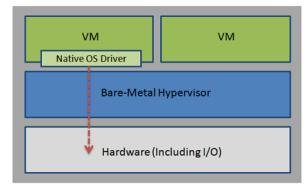
Figure 5. Bare-Metal virtualization software can enable I/O devices to be partitioned amongst individual virtual machines for direct access.
