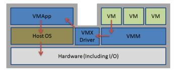
Figure 2. Hosted virtual machine monitor (VMM) software is typically made up of different components that all communicate to channel virtual machine (VM) I/O requests through the host operating system (OS).
