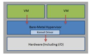
Figure 4. In the bare-metal virtualization architecture, system I/O devices that are shared between virtual machines must be accessed by a kernel driver that is part of the hypervisor.
