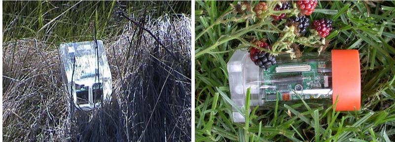
Figure 18.3. Acrylic enclosures used at different outdoor applications.
