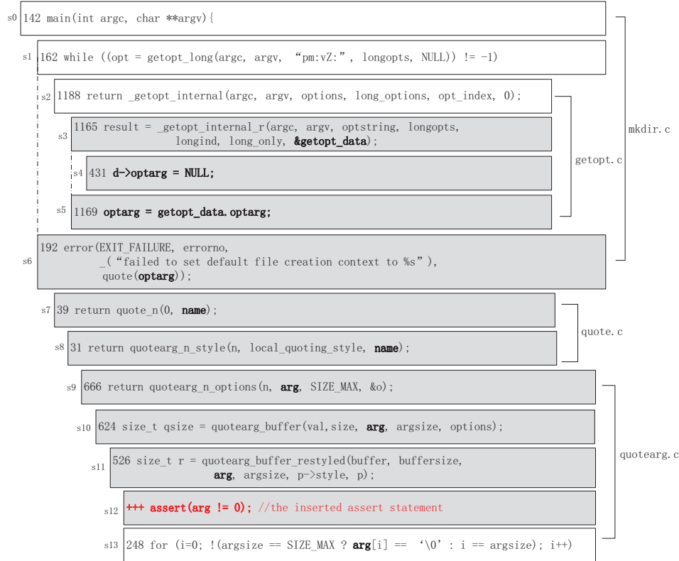
Fig. 11. The root cause of the failure in mkdir under the command ' mkdir -Z a b '.
